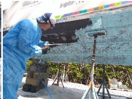
Spray the Bare Bottoms on in a thick layer
