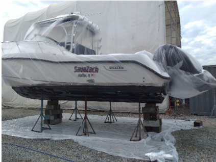
Cover topsides and under the boat with plastic
