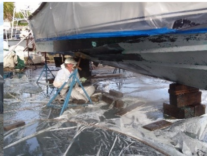
Make sure boat is high enough to spray on and pressure wash off
